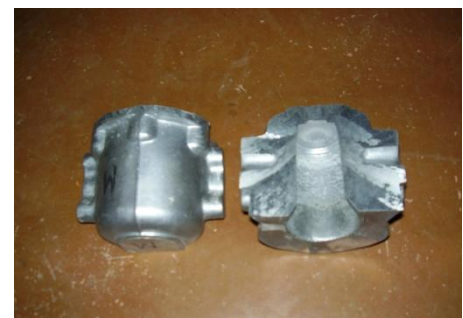
Fig. 2. Appearance of industrial casting from aluminum alloy AK5M, modified (with the letter "M") and control serial (with the letter "K"):
