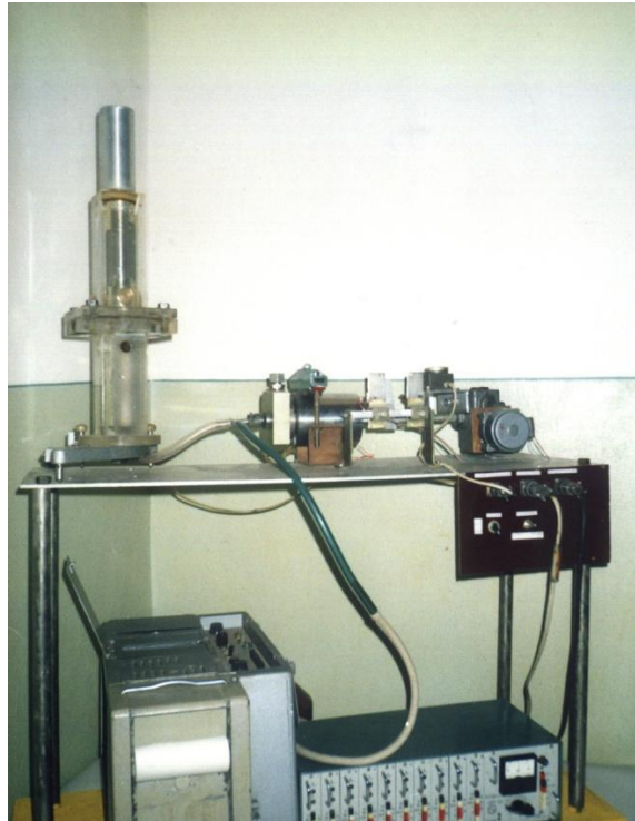
Fig.4. General view of the experimental setup for the study of the hydraulic resistance of mesh phase separators in non-stationary liquid flow
