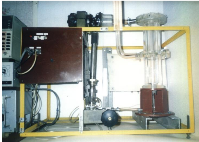
Fig.2. General view of the experimental setup for the study of the interaction of gas bubbles with a mesh phase separator
