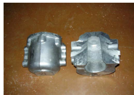
Fig. 2. Appearance of industrial casting from aluminum alloy AK5M, modified (with the letter "M") and control serial (with the letter "K"):
