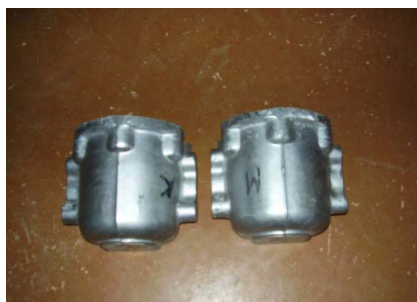
Fig. 2. Appearance of industrial casting from aluminum alloy AK5M, modified (with the letter "M") and control serial (with the letter "K"):
