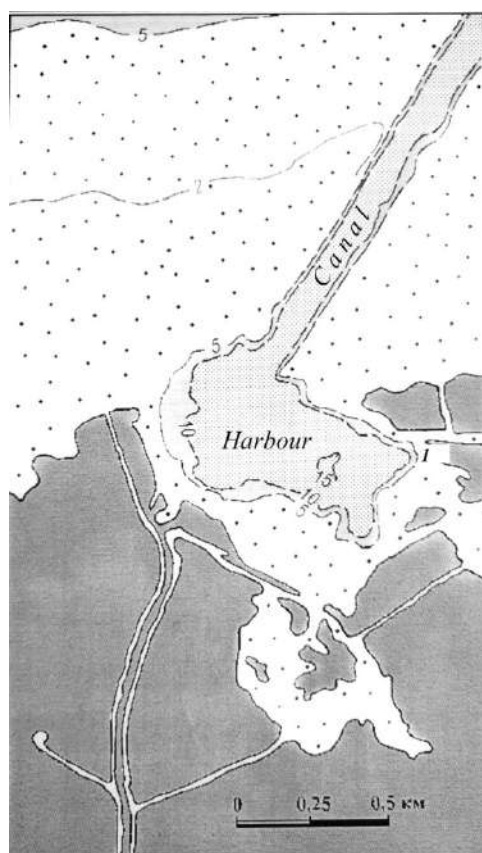
Fig. 7. Scheme of the port harbor of Ust-Danube and the approach channel to it. A dark fill indicates the Danube Delta; 1 – the beginning of the technical channel.
