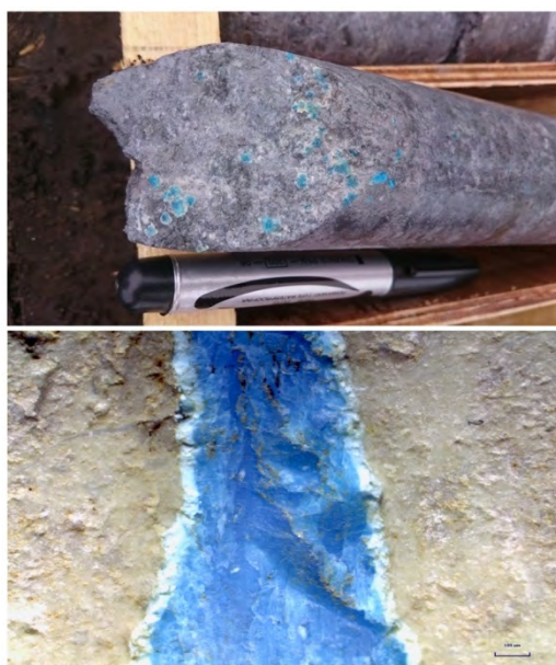
Fig. 8. Turquoise ( \text{CuAl}_6(\text{PO}_4)_4(\text{OH})_8 \cdot 4\text{H}_2\text{O} ) mineralization in the Reza gold deposit: turquoise minerals observed on fractures, rhyodacite core piece (the upper); turquoise mineral fragment in rhyodacite rock, photos taken under Leica S8AP0 Binoculars (the following).
