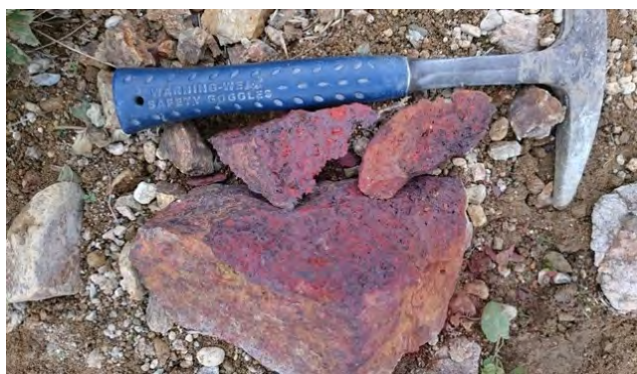
Fig. 9. Hematite mineralization, oxide zone: Left side-hematite vein on andesite porphyritic fractures and Right side- barite veinlets oxidation secondary quartzite.
