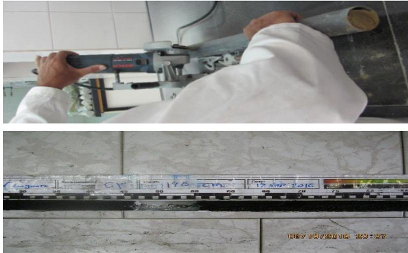
Fig. 3. Cutting of polyethylene pipes by means of milling machine (above) and sedimentary cores after cutting (below)
