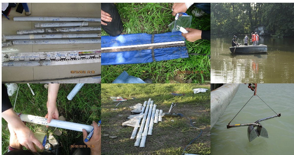
Fig. 2. Coring the wetland using polyethylene pipes, and packing and recording the cores (left), and sampling by grab (right)
