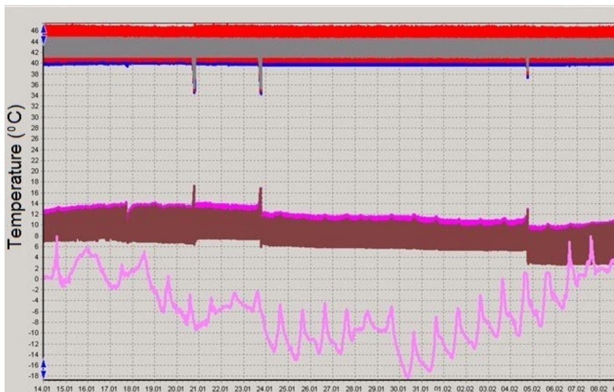
Fig. 6. Curve for input and output temperatures on the condenser and evaporator of the heat pump geothermal system versus the load on the soil collector
