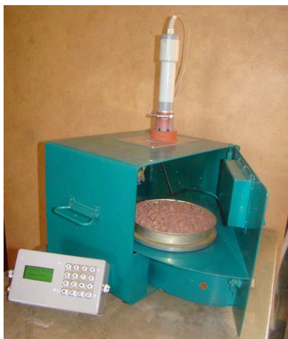
Fig. 15. Integrated device for controlling the total iron content PAKS-5 M
