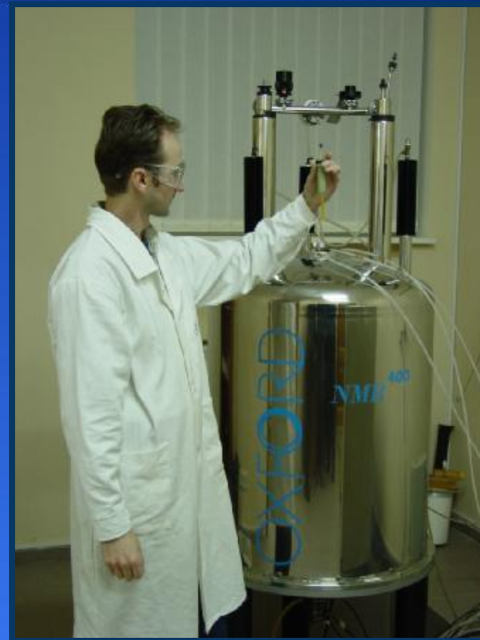
Varian INOVA Plus 400 MHz NMR spectrometer
