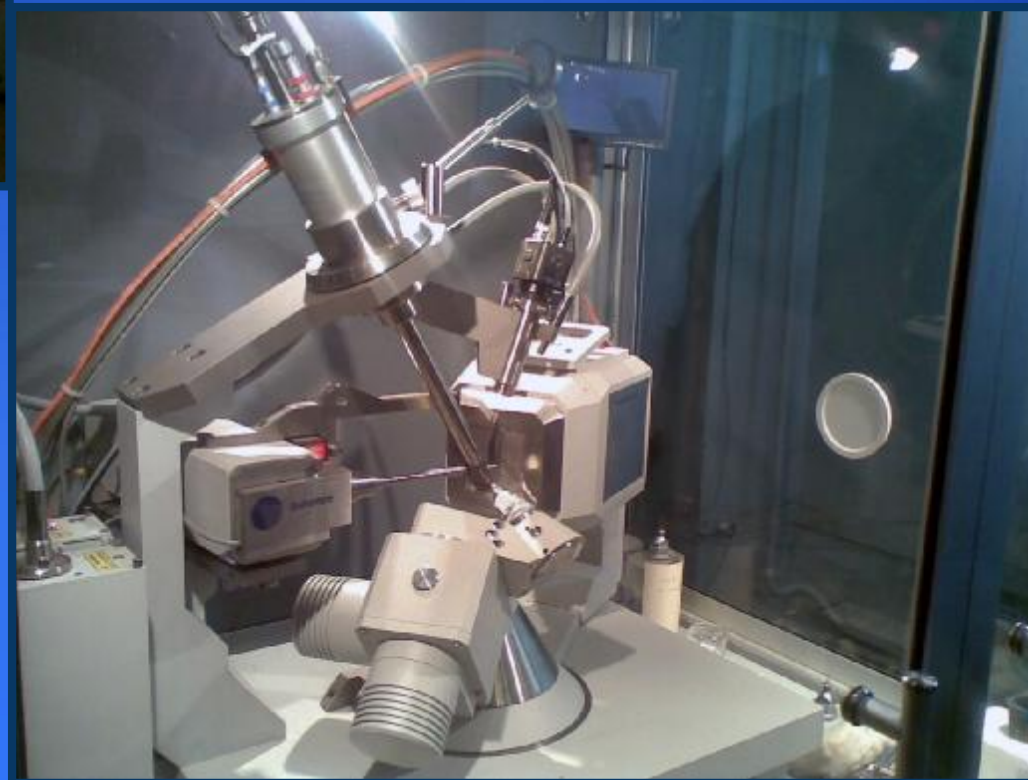
Xcalibur-3 X-ray analysis
